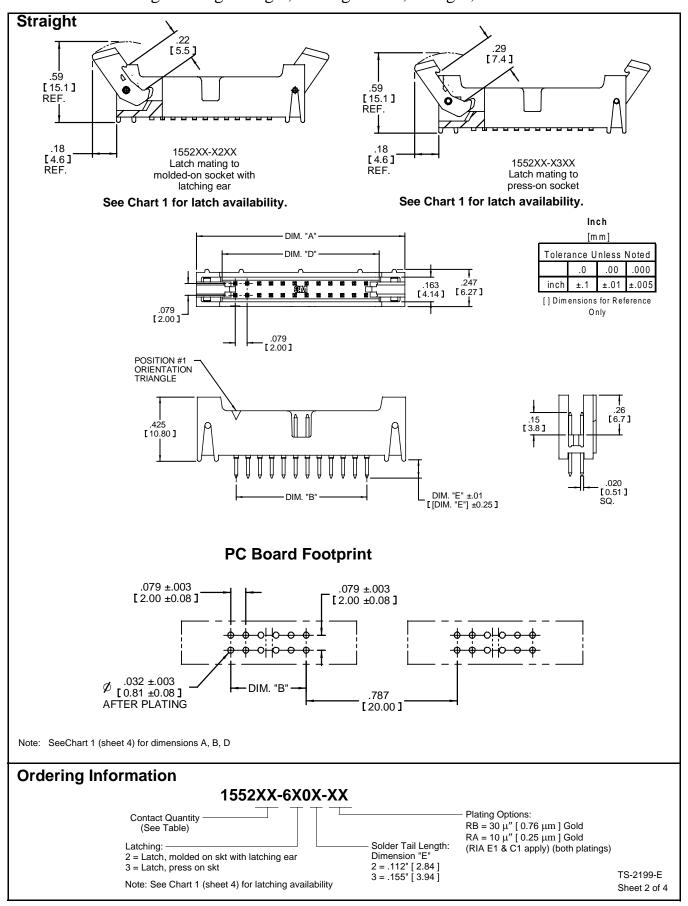
2 mm x 2 mm Straight & Right Angle, Through-Hole, Straight, Surface Mount 1552 Series
