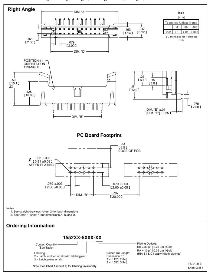
2 mm x 2 mm Straight & Right Angle, Through-Hole, Straight, Surface Mount 1552 Series
