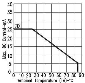
Fig5. MAX. ALLOWABLE DC CURRENT VS. AMBIENT TEMPERATURE.
