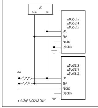
Figure 8. Typical I<sup>2</sup>C Application Circuit
