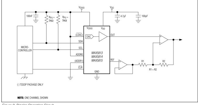
Figure 9. Bipolar Operating Circuit
