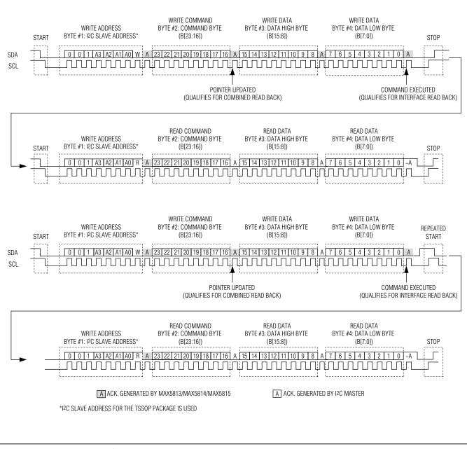
Figure 7. Interface Verification I<sup>2</sup>C Register Read Sequences
