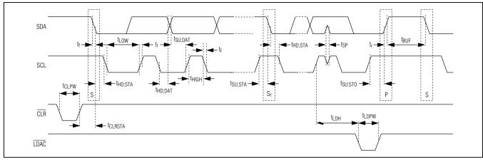
Figure 1. I<sup>2</sup>C Serial Interface Timing Diagram
