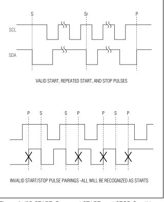
Figure 2. I<sup>2</sup>C START, Repeated START, and STOP Conditions
