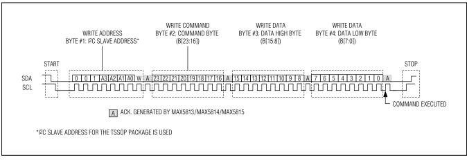
Figure 4. I<sup>2</sup>C Single Register Write Sequence
